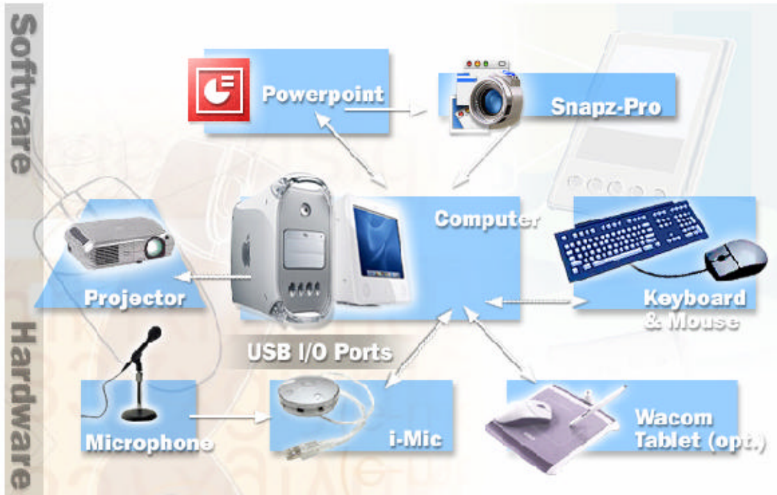
Figure 1. Hardware and Software Diagram for Recording Lectures
